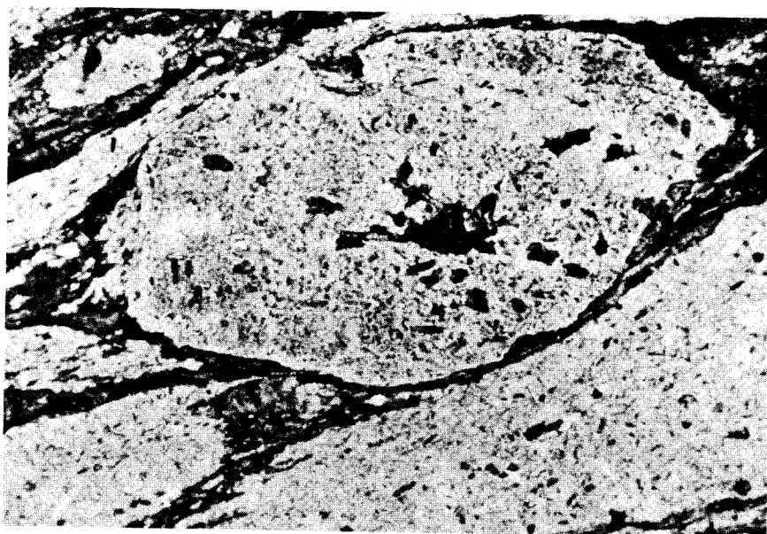
Figure 7. Photomicrograph of fragmental metavolcanic. Plagioclase fragment elongated along biotite-rich shears in an accumulation of squashed lapilli. Width of field approximately 3.5 mm.
